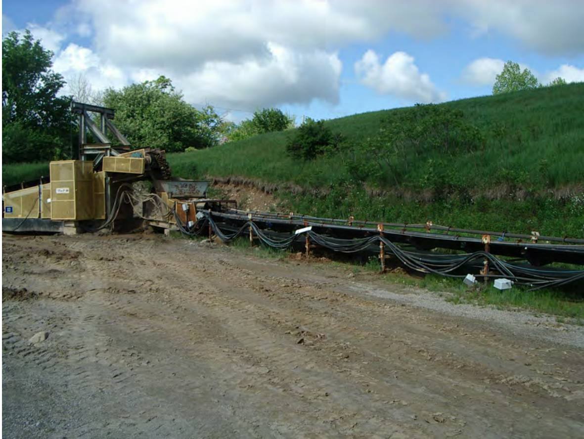
Photo 7: Conveyor on the north side of Concession Road 2. This conveyor has moved aggregate material from Phases 2 and 6 of the Mill Creek Pit and the adjacent McMillan Pit to the Mill Creek processing plant. This portion of the berm and yard are outside of the proposed SPA extraction area. GEC 2022-05-28
